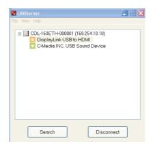
Double click on the GREEN sign, the system will connect the devices and after connect successfully it will turn to ORANGE sign. When connect other devices with USB port, "Launch USB Server" will detect it and show out a GREEN sign. Double click the GREEN sign to connect the device(s) in order to activate and use it.
